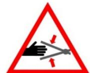
**Caution:** Failure to observe this instruction may lead to trapping of the hand and fingers.
